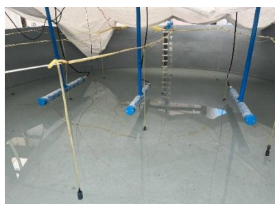
Mangrove crab larval rearing set-up with the inclusion of water heaters
