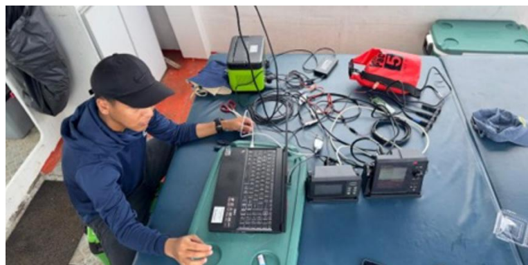
Coastal fisheries acoustic surveys using the portable echo sounder” Furuno FCV600” from August to November 2025 in the west coast of Malaysia
