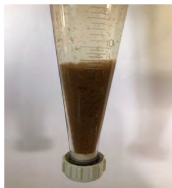
Settleable solids from one of the treatments
