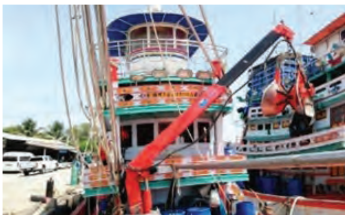
Figure 2. Installation of hydraulic machinery (crane and power block)
