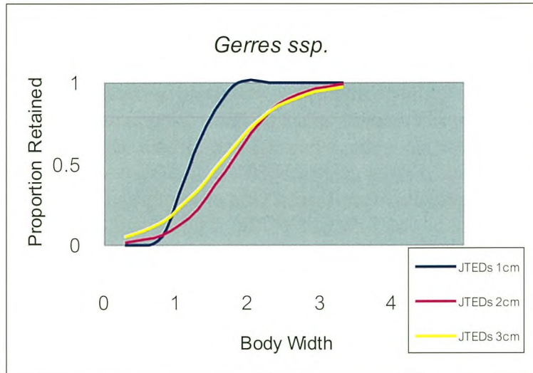
Figure 16. The selectivity ogive of Gerres ssp. in body width from the trawl net using 1, 2 and 3 cm bar spacing rigid sorting grid JTEDs.
