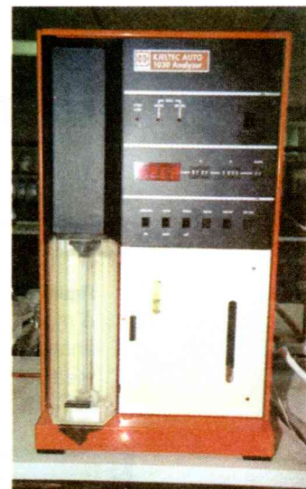
Figure 6.3 The Kjeldahl distillation-titration (Kjeltec™) apparatus used to analyze crude protein.
