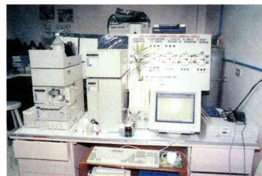
Figure 6.7 The high performance liquid chromatograph (HPLC) used for analysis of amino acid composition of a protein.
