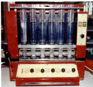
Figure 6.6 The Fibertec™ used for crude fiber determination.
