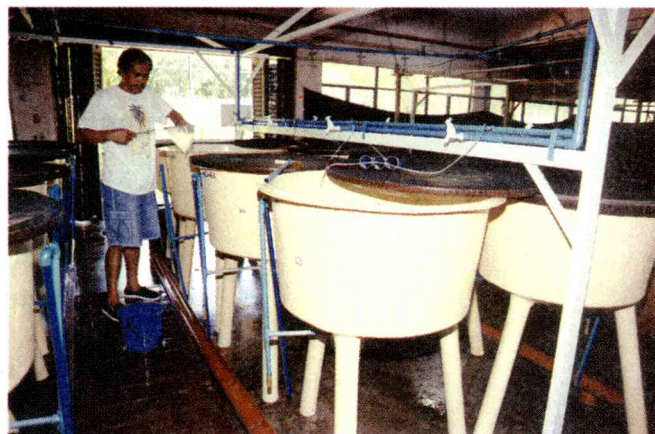
Figure 6.11 A laboratory set-up for a feeding experiment using 250 l tanks.
