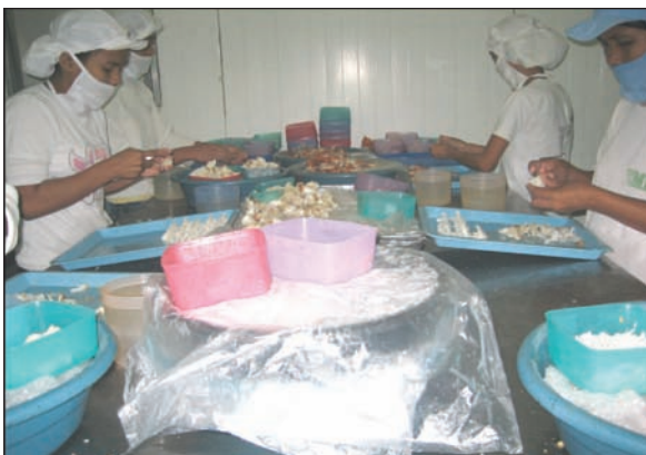
Figure 12. Picking of crab meat into coded containers placed in a bed of ice.
