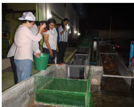
Experiment on fish migration behavior at 5, 8, 11-degree slope design of the vertical-slot fishway during night time
