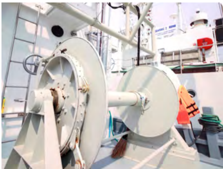
Net drum installed at the rear part to reduce the number of crew involved in fishing operations
