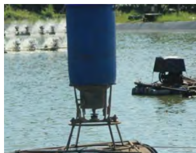
Figure 6. Auto-feeding system in operation in intensive shrimp farm in Thailand
