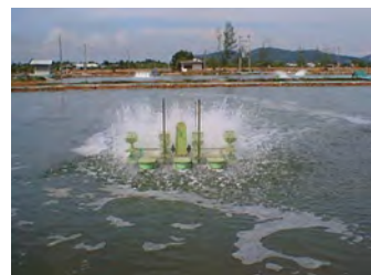
Figure 10. Typical 4-wheel aerator
