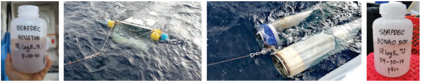
Figure 16. Nueston net (left) and bongo Net (right)
