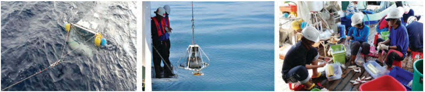
Figure 19. Study on microplastic accumulation in the Gulf of Thailand (from left to right): collection by neuston net; collection by Smith McIntyre grab; and data on marine biota based on dominant and economically important fishes
