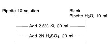
Titrate with 0.05N Na<sub>2</sub>S<sub>2</sub>O<sub>3</sub> with starch indicator
