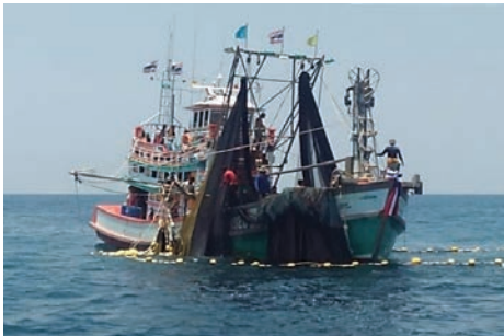
Thai traditional purse seine fishing vessel hauling the net from both sides, port and starboard sides with nearly 40 crew members onboard (before installation of modern fishing machinery)
