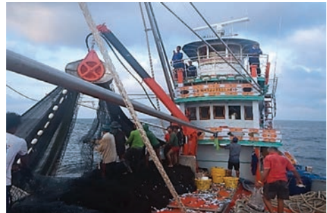
Thai purse seine fishing vessel hauling net only from starboard side with only 16 crew members onboard after installation of modern fishing machinery, e.g. hydraulic crane, power block and refrigeration seawater cooling system (RSW) with modification of the net plan
