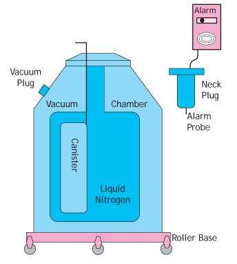
**Figure 3.** Diagram of a liquid nitrogen storage dewar (with permission from Wayman and Tiersch).
