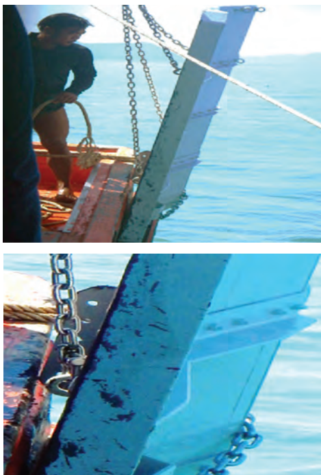
Figure 5. Fewer scratches on the painted footer plate of the V-shaped otter board of M.V. Plalung
