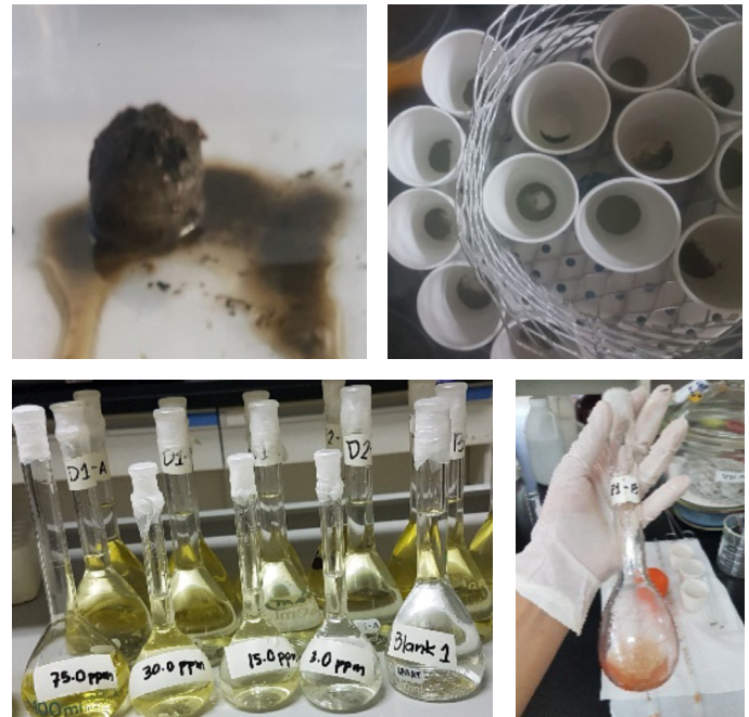
Figure 6. Chromic oxide analysis of feeds and feces for digestibility study (clockwise: thawing of collected frozen species; ashen feeds and feces samples; concentrated digested sample; and diluted digested samples for spectrophotometer reading)
