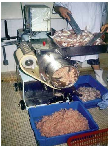
Some examples of low-cost fish processing equipment (left to right): meat-bone separator, silent cutter, fishball forming machine
