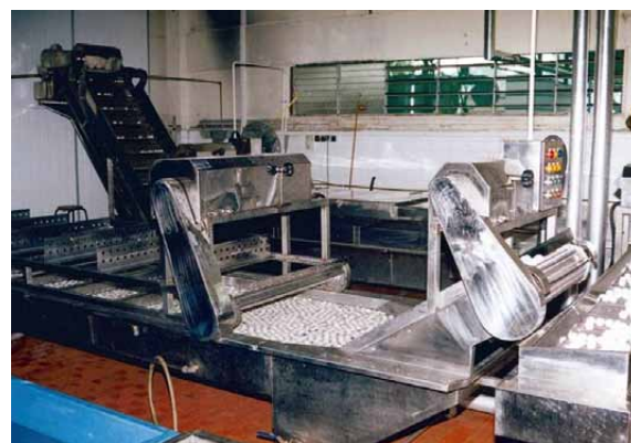
Automated systems for fish processing: chikuwa processing (above), imitation crab stick processing (right top), and fish ball processing (right)
