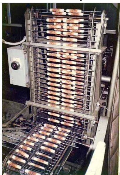
Automated systems for fish processing: chikuwa processing (above), imitation crab stick processing (right top), and fish ball processing (right)
