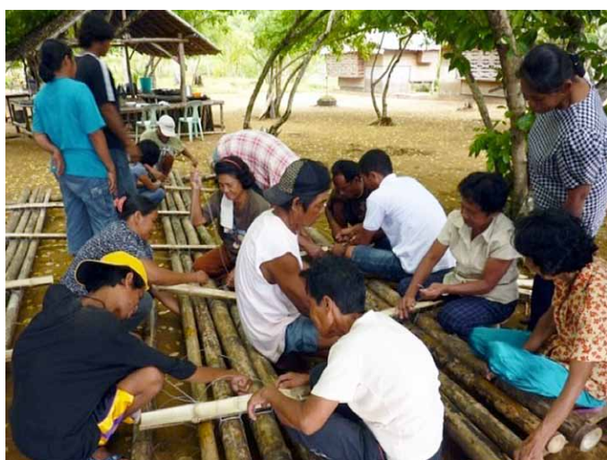
Project collaborators in Guimaras construct fish cages for milkfish culture using bamboo frames
